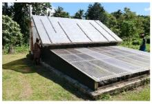
Their drier is a combo sun and fire system. In an effort to manage the capital outlay, the group uses a combination of UV-resistant polyvinyl sheeting and polycarbonate sheets. Black stones for storing heat can been seen in the photo.
