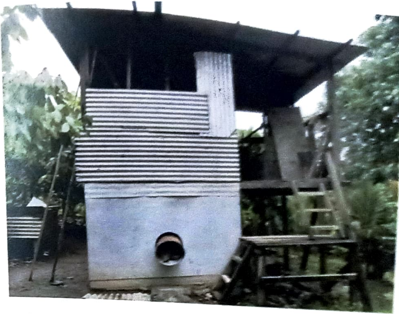
Figure 11.4: The most commonly used fire wood based energy drier.
